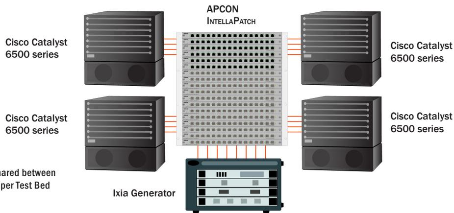
**Figure 2.** Ixia generator shared between a pool of devices in the Super Test Bed
