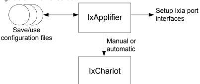
IxApplifier is run first in order to setup the Ixia port interfaces. IxApplifier configurations may be saved and later re-used. After setting up the ports, IxApplifier may be configured to automatically start IxChariot.
