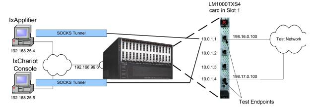
In Figure 3-4, the two PCs independently use SOCKS to create a tunnel from their network interface to the management address for the Ixia ports *through* the interface on the Ixia chassis (192.168.99.6). The SOCKS server on the Ixia chassis forwards the tunneled packets to the port interfaces.
