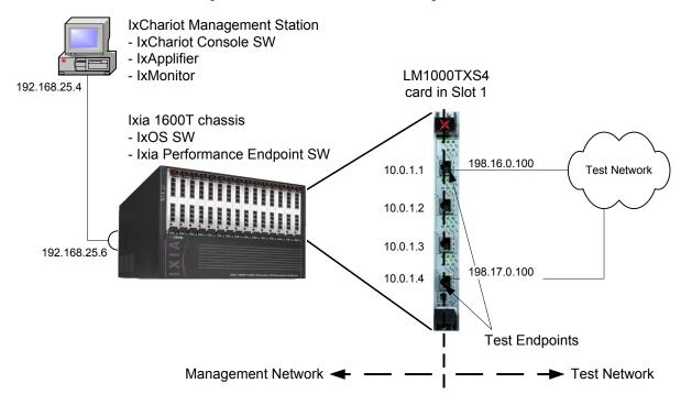
This configuration logically divides the management network from the test network. The management network includes the IxChariot Management Station, Ixia chassis and the management addresses associated with the ports (10.0.1.1-10.0.1.4 in the figure. The test network contains the network components which are part of the test network (198.\*.\*.\*\* in the figure).
